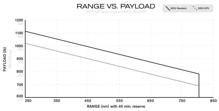
+1 lb (.45kg) Payload or Equipment = -1.7 NM 75% to 55% PWR = +40% Range
